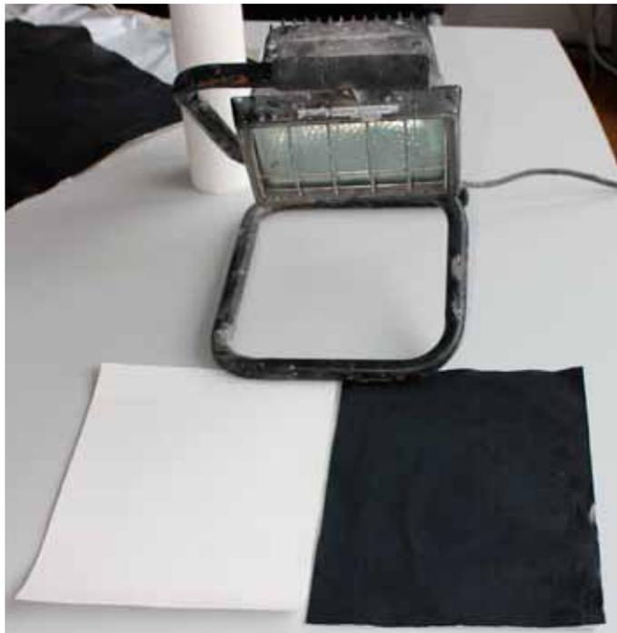
**Picture above: Test setup for heat reflection of KÖSTER 21.**
